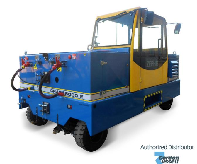
MAXIMUM DRAWBAR PULL: 11,690 lbf (52 kN) WEIGHT: 19,850 lbs (9.9 US t) DIMENSIONS LxWxH: 151.6"x86.6"x104.3" (3850 mm x 2200 mm x 2650 mm) UNLOADED RAIL SPEED: 4.9 mph (7.5 km/h) RAIL SPEED AT MAX LOAD: 1.8 mph (2.75 km/h) STANDARD GAUGE: 56.5" (1435 mm)
